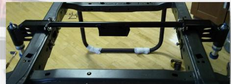
8. Locate the large triangular frame support assembly. Place the assembly under the truck with the wide end facing the rear. From under the frame place the assembly against the top plate of the cross member from step 7.
