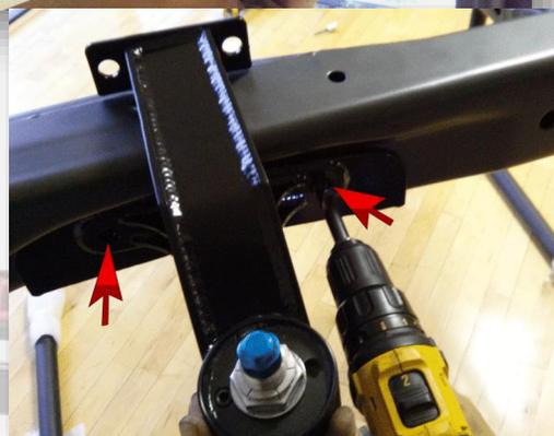
4. Use the 4 1/2" x 1/2" Grade 8 Bolts to go through the bump stop bracket assembly, the side frame gusset plate, and through the stock frame. Place one 1/2" washer on the bolt and insert from the outside inward.
