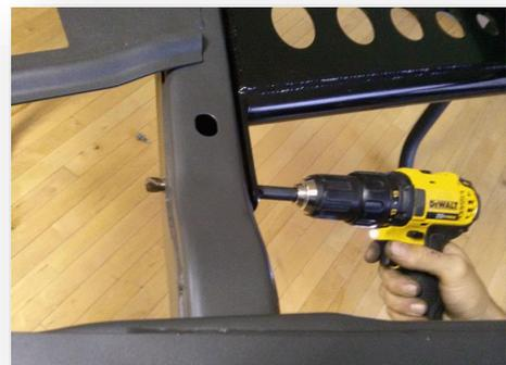
11. Locate the 4 holes in the rear larger side of the triangular frame support. Again, take the 90' drill and ½" drill bit and drill through the stock cross member. Install 4½" x ½" Grade 8 Bolts to secure the triangular frame support to the stock cross member. Make sure you use washers and put the nuts on the threaded end of the bolt.
