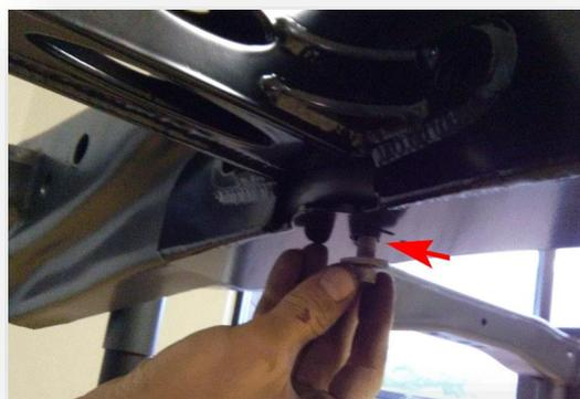
3. Using the Bump Stop Assemblies as a template, drill a 1/2" hole through the frame gusset and into the inside portion of the stock frame. Pay attention to drill as straight as possible.
